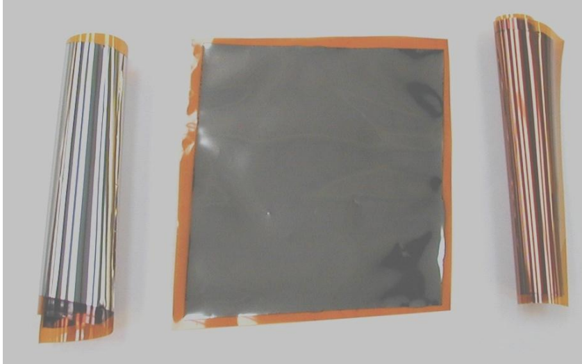
Figure no. 19 : it is possible to deposit within compression or tension through a zero stress.
